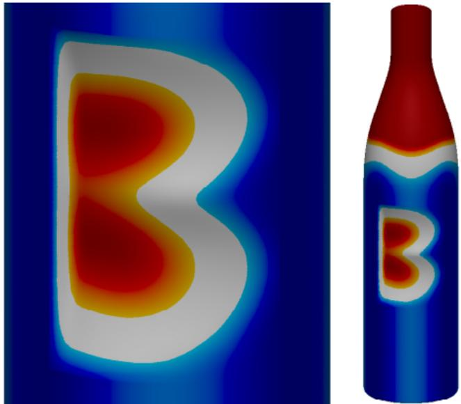
hierarchical basis: two levels, 52 + 209 B-splines
